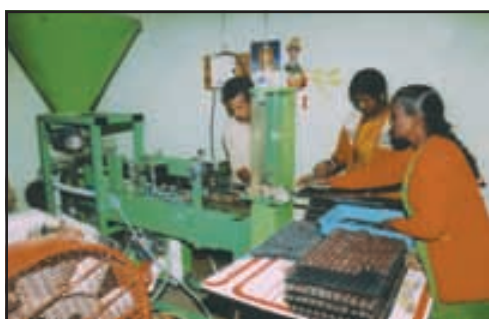
Plug Making machine used for making rooting bags for carnation seedlings (TN)
